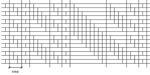
**Figure 1: Bitonic sorting networks for 16 elements. Each step is completed when all comparisons involved are computed. In the figure each comparison is represented with a vertical line that link two elements, which are represented with horizontal lines.**
